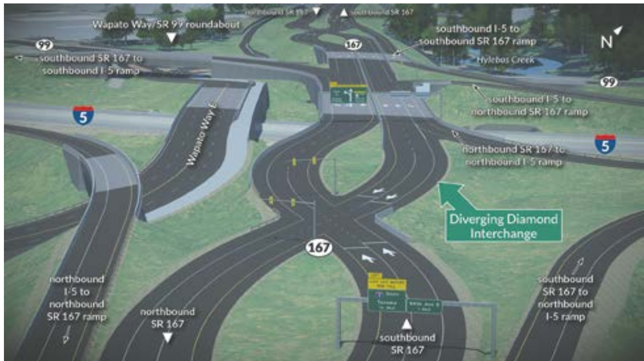
The state Route 167 Completion Project will build a new diverging diamond interchange, or DDI, at I-5 creating direct connections between I-5 and SR 167. WSDOT will build half of the DDI, including the southbound SR 167 to southbound I-5 on-ramp, by 2026; the remaining ramps will be completed and open to traffic by 2029.
